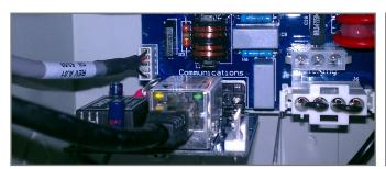
Figure 2: Connection to the PVP 1010 network card with standard ethernet cord.
