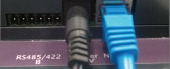
**Figure 3**: Connection to the STL 200/400. Blue ethernet cord is connected to ethernet switch.
